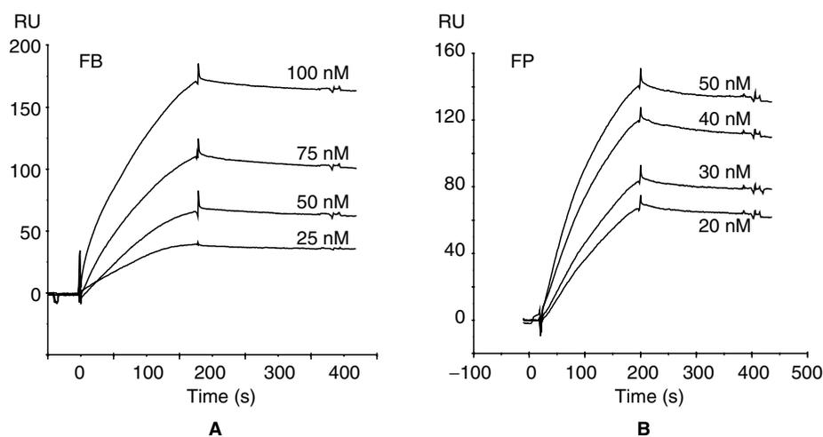
**Figure 18** SPR sensorgrams of interaction between factor B (A) at 12.5, 50, 75, and 100 nM; factor P (B) at 20, 30, 40, and 50 nM, with biotinylated heparin immobilized on a poly(ethylene glycol) (PEG)-based chip.
