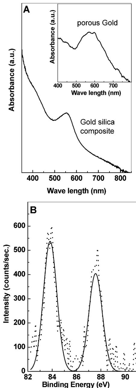
**Figure 1.** (A) UV-vis spectra of the silica-gold composite before and after (inset) treatment with HF. (B) Au 4f core-level spectra recorded from a porous gold nanoparticle film deposited on a copper substrate. The spin-orbit components are shown.
