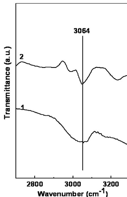
**Figure 3.** FTIR spectra of a drop-coated film of silica-gold composite particles (curve 1) and porous gold nanoparticles (curve 2) on a Si(111) substrate.
