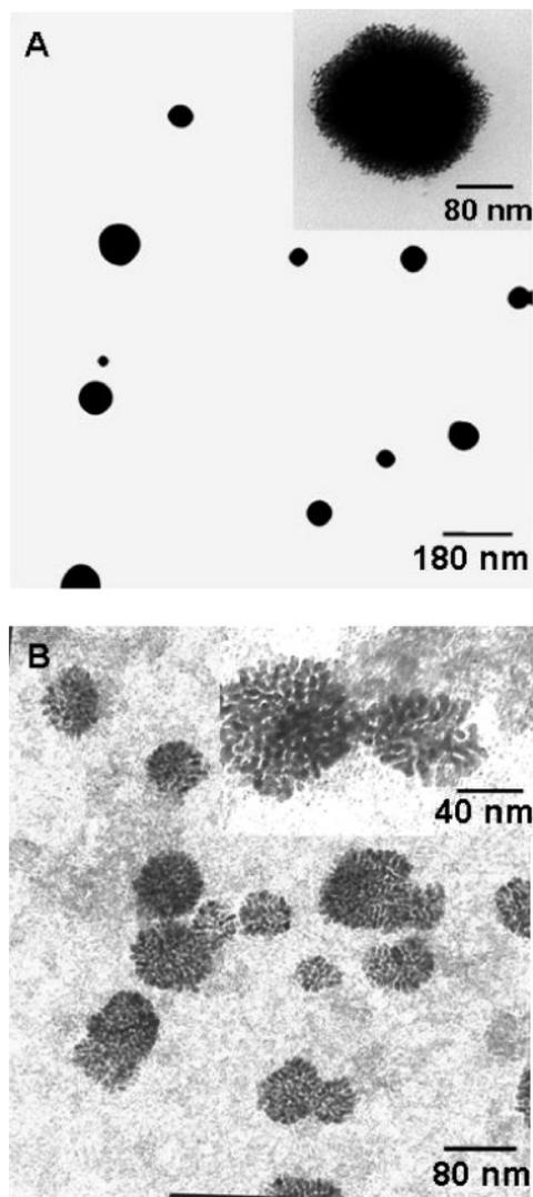
**Figure 4.** TEM image of a drop-coated film of a silica-gold composite (A) before and (B) after HF treatment on a carbon-coated copper grid.
