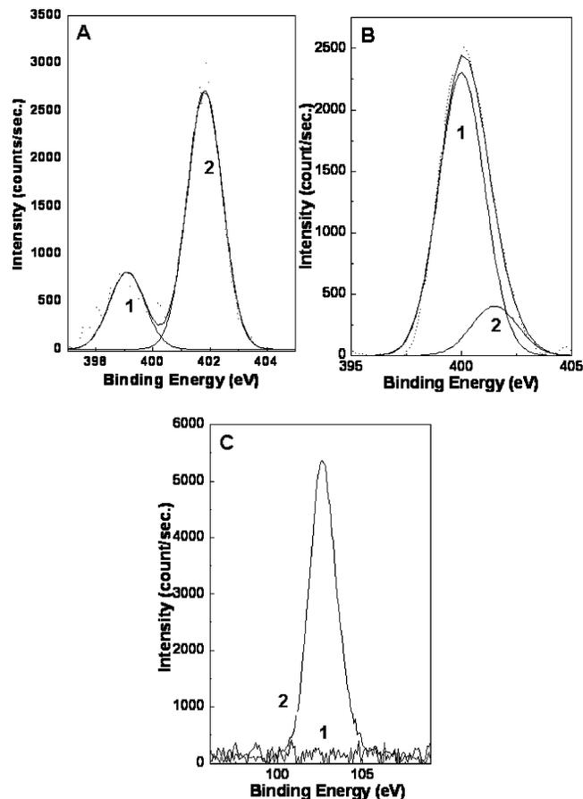
**Figure 2.** (A) N 1s core-level spectra recorded from a porous gold nanoparticle (A) and a silica-gold composite film (B) deposited on a copper substrate. (C) Si 2p core-level spectra recorded from a porous gold film (curve 1) and a silica-gold composite film (curve 2) deposited on a copper substrate.
