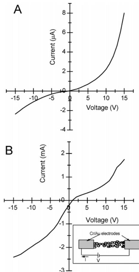
**Figure 5.**  $I$ - $V$  curves of (A) a silica-gold composite and (B) porous gold nanoparticles measured at 300 K. The inset shows a schematic of metal electrodes with nanoparticles or composite dispersed between the electrodes.
