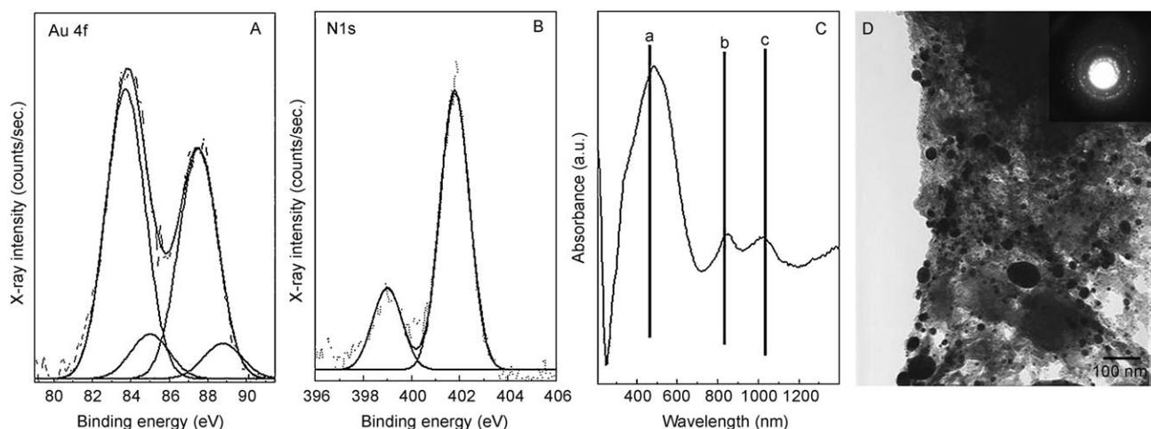
**Figure 2.** A, B) Au 4f and N 1s core-level spectra recorded from a Au–RTIL film grown on a Si(111) substrate. C) UV/Visible spectrum obtained from the drop-coated film of rods. D) Transmission electron microscopy (TEM) image of a drop-coated film of the Au–RTIL solution on a carbon-coated grid (inset: diffraction pattern of gold).
