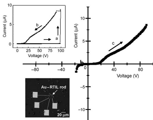
**Figure 5.** Current–voltage ( $I$ – $V$ ) characteristics of a single hexagonal Au–RTIL rod obtained from the second scan onwards. The top inset shows the  $I$ – $V$  curves obtained during the first scan forth and back. The bottom inset shows the SEM image of the Pt electrodes deposited on the Au–RTIL rod. The square pads are the Pt electrodes.
