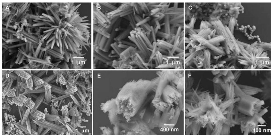
**Figure 3.** Growth mechanism of anisotropic hexagonal organic-metallic nanorods.
