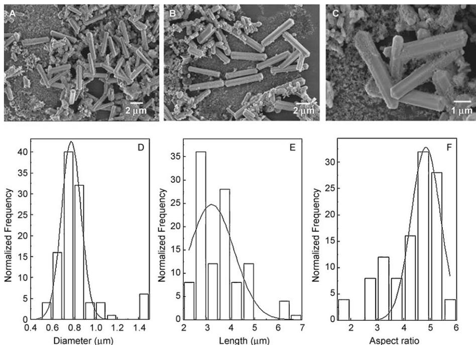
**Figure 1.** A–C) SEM images of Au–RTIL rods obtained with ionic liquids. D–F) Size distributions of the rods shown in A–C, respectively.
