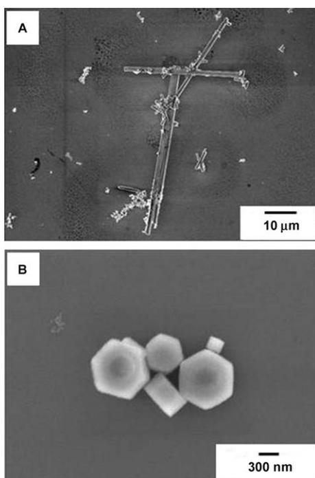
**Figure 4.** SEM images of hexagonal rods obtained by using an ionic liquid at A) 1:4 molar ratio and B) 1:130 molar ratio.
