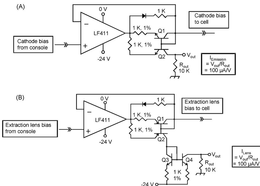
**Fig. 1.** (A) Analog circuit designed to measure the emission current of the EDD cathode. Q1 and Q2 are a matched pair of npn transistors. (B) Analog circuit designed to measure the extraction lens current. Q1/Q2 are a matched pair of pnp transistors, and Q3/Q4 are a matched pair of npn transistors. The electron current sourced by the cathode and sunk by the lens are mirrored and converted to a voltage by 10 K resistors.
