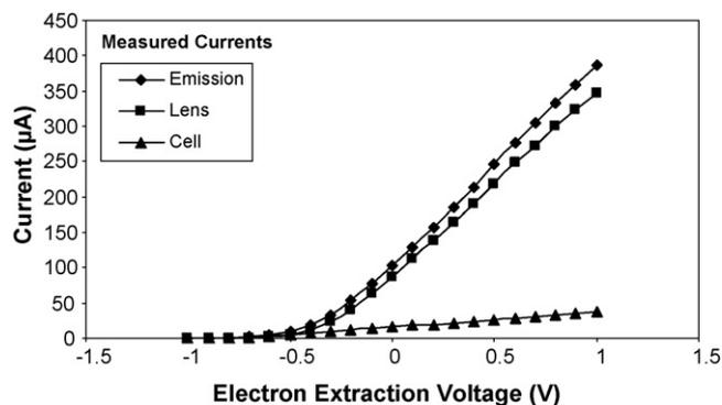
**Fig. 2.** Electron currents ( $\mu\text{A}$ ) as a function of the potential difference between the extraction lens and dispenser cathode,  $\Delta V$ , at a heater current of 1.6 A. A sub-optimal transmission efficiency is observed for electrons entering the FTICR analyzer cell.
