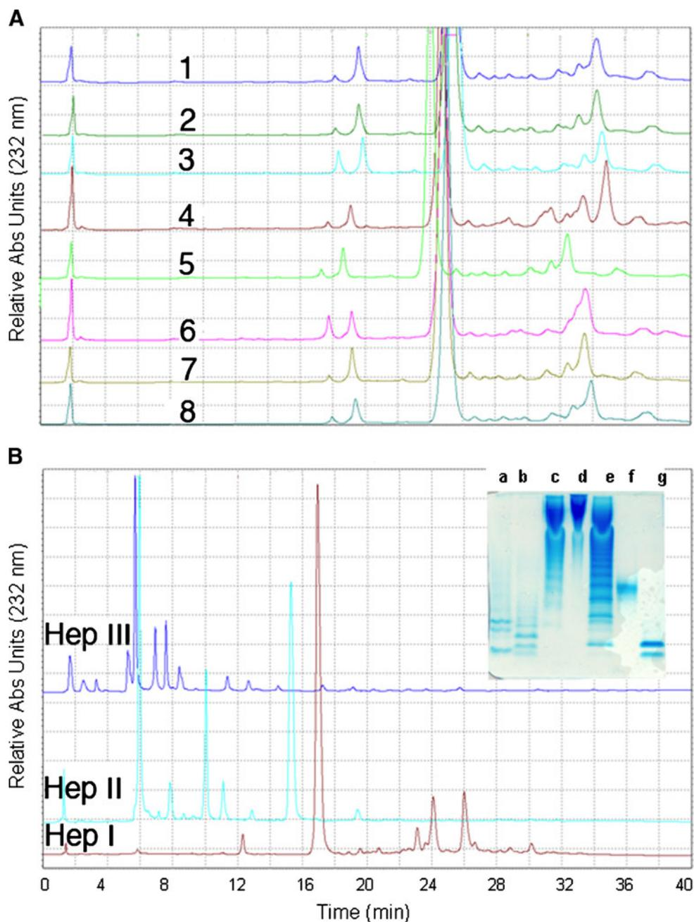
**Table 5** SAX-HPLC analysis of seven commercial heparin samples digested with Hep I, II, or III
