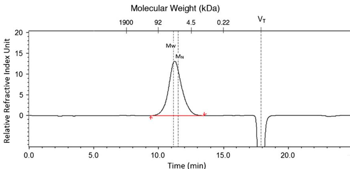
**Fig. 2** A sample chromatogram using SEC for heparin molecular weight determination of heparin no. 1. The y-axis corresponds to the mass detected using a refractive index detector, and the x-axes
