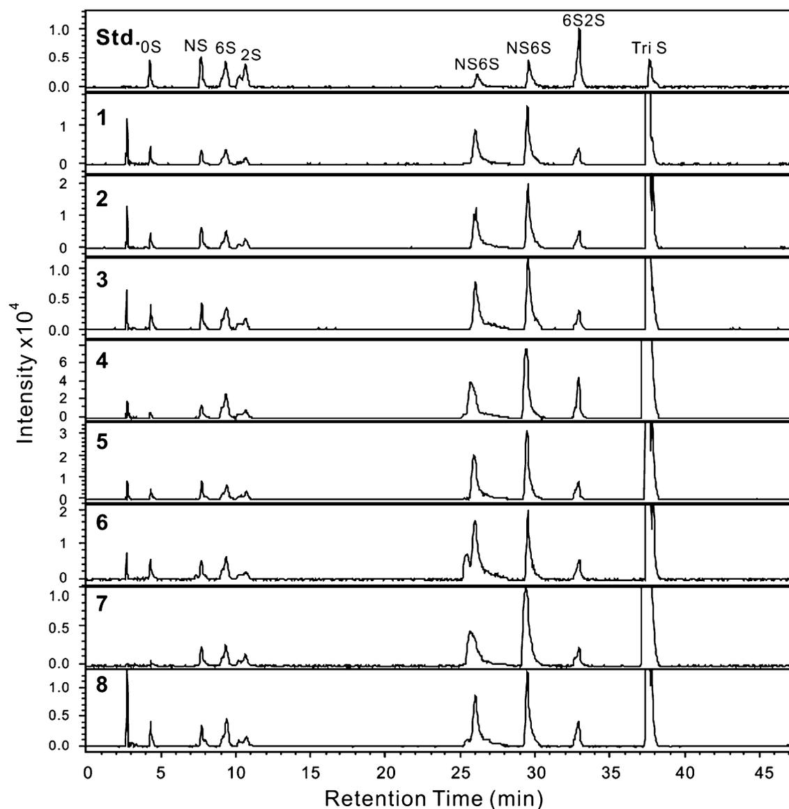
**Fig. 3** EIC of disaccharide analysis of seven heparin samples and one LMWH sample by RPIP-UPLC-MS. *Std* shows the analysis of an equimolar mixture of eight disaccharide standards used for peak identification and injection of different amounts afford a standard curve for quantification. Chromatograms 1–8 show the disaccharide
