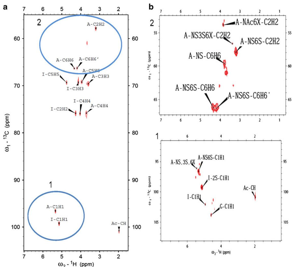
**Fig. 6** Two-dimensional  $^1\text{H}$ - $^{13}\text{C}$  correlation spectrum (HMQC) of heparin no. 1. **(a)** Entire HMQC spectrum. **(b)** The selected regions of the spectrum. Blue circles 1 and 2 indicate anomeric region and H2/C2-H6/C6 glucosamine resonances, respectively
