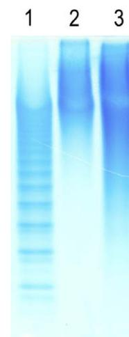
**Figure 2.** PAGE analysis of HP and CR-HP. Lane 1 shows a ladder of heparin oligosaccharide standards,<sup>17</sup> lane 2 is HP and lane 3 is CR-HP.
