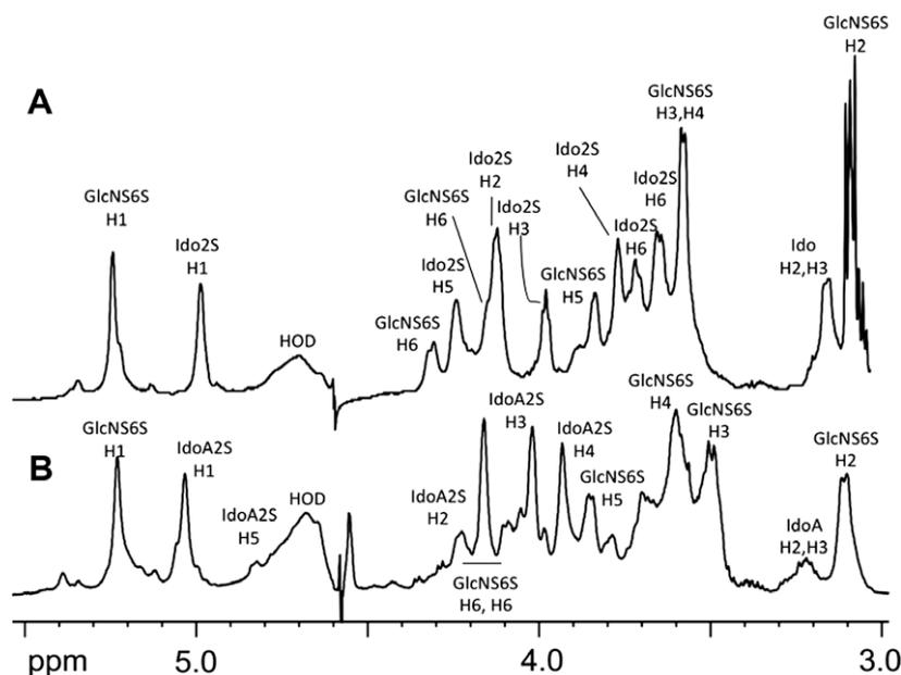
**Figure 3.** Expanded  $^1\text{H}$  NMR spectra from 3 to 5.5 ppm of (A) CR-HP and (B) HP at 500 MHz and 300 K. Signals are labeled based on assignments made using 2D NMR spectroscopy.
