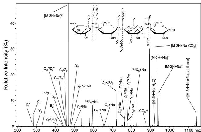
**Figure 3.** NETD of the  $[M - 3H + Na]^{2-}$  precursor ion of Structure **1** using fluoranthene as the radical cation. Products assigned to the observed fragmentation are shown in the inset. Selection of a precursor ion in which all sulfates are ionized or paired with a Na minimizes the loss of  $SO_3$ .
