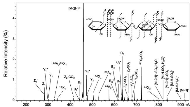
**Figure 4.** NETD of the  $[M - 2H]^{2-}$  precursor ion of Structure **1** using xenon as the radical cation. Products assigned to the observed fragmentation are shown in the inset. Although the use of xenon as a reagent gas increases the number of cross-ring cleavages observed,  $SO_3$  loss is also increased.
