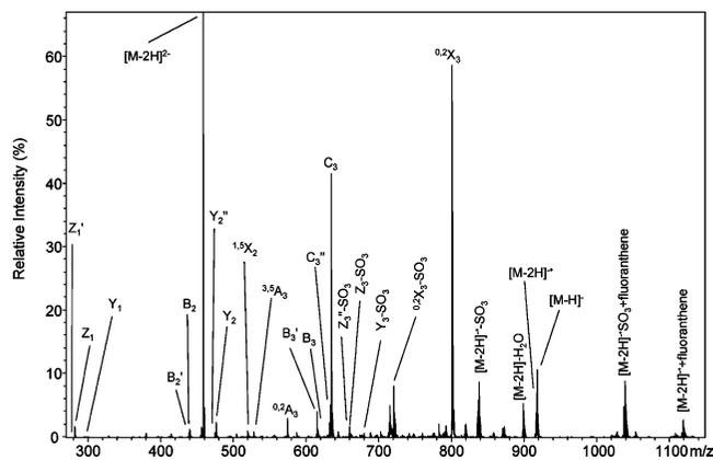
**Figure 1.** NETD of the  $[M - 2H]^{2-}$  precursor ion of Structure **1** using fluoranthene as the radical cation. The NETD spectrum demonstrates abundant glycosidic and cross-ring bond cleavage, similar to the published EDD for the same precursor ion.
