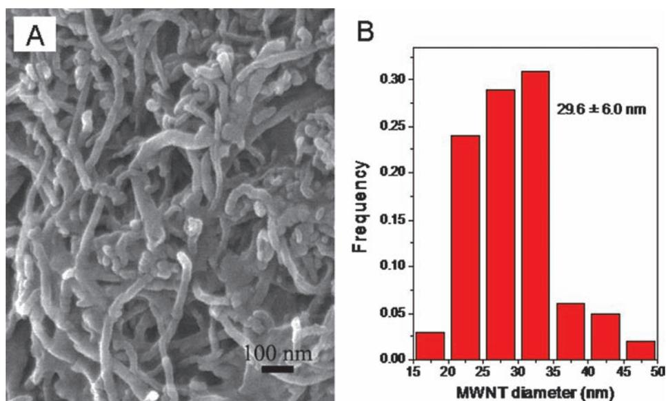
**Fig. 1.** SEM image (A) and size distribution (B) of as received MWNTs. The average size of as received MWNTs is 29.6 nm with 6 nm as standard deviation.
