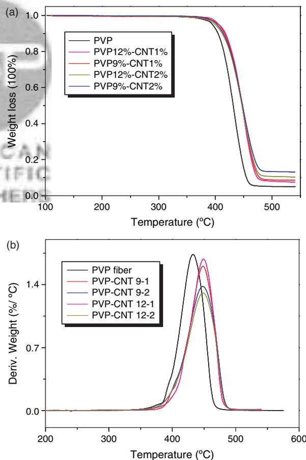
**Fig. 3.** Thermalgravetric analysis (TGA) of PVP-MWNTs core sheath fiber mats.
