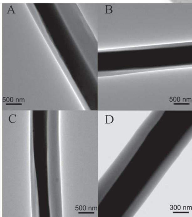
**Fig. 5.** Bright fields of TEM images, from (A) to (D) PVP-MWNTs 9-1, 9-2, 12-1 and 12-2.
