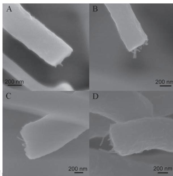
**Fig. 6.** SEM images of fiber cross-section from (A)-(D) PVP-MWNTs 9-1, 9-2, 12-1, and 12-2.
