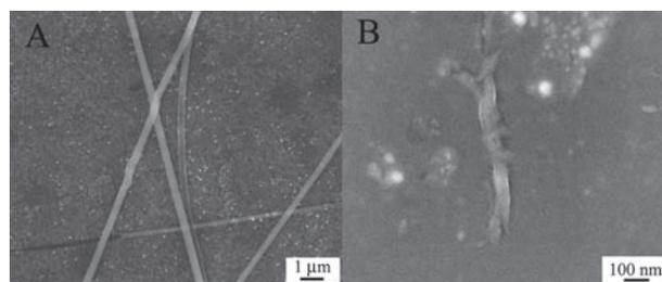
**Fig. 7.** SEM images of fiber etching with isopropanol vapor, (A) before and (B) after etching with isopropanol vapor at room temperature.
