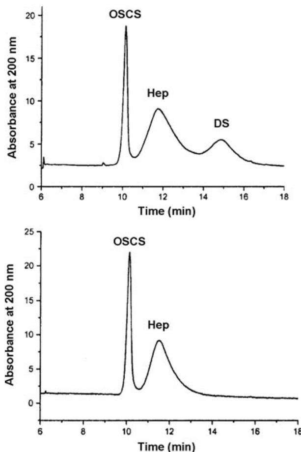
**Figure 2.** CE-UV of OSCS-contaminated heparin samples (modified from [31]). Sample concentration: 50 mg/mL. Capillary id: 25  $\mu\text{m}$ . Total capillary length: 60 cm. Buffer: 850 mM Tris-phosphate pH 3.0. Capillary temperature: 35°C. Sample injection: 48 s at 2.0 psi. Voltage: -30 kV. Voltage ramping time: 5.0 min.
