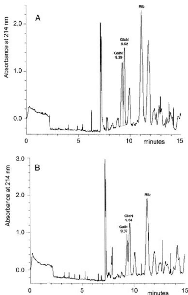
**Figure 4.** CE electropherograms at 214 nm of glucosamine (GlcN) and galactosamine (GalN) derivatized with anthranilic acid and obtained after hydrolysis procedure of (A) a contaminated raw heparin or (B) a formulated contaminated heparin sample. Ribose (Rib) is used as an Internal Standard. Modified with permission from [33].
