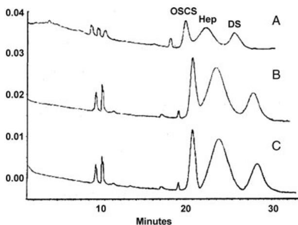
**Figure 3.** Electropherograms of OSCS, heparin, and DS under different background electrolyte. (A) 400 mM Tris-phosphate pH 3.5, (B) with 0.5% polymeric- $\beta$ -CD, and (C) with 0.5% polymeric- $\beta$ -CD and 0.4% Tetric<sup>®</sup> 1107. Modified from [32].
