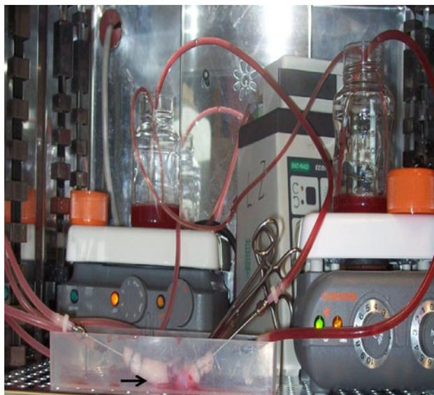
**Fig. 1** Perfusion system showing the recirculation of pancreatic cells through the cannulated vein of human umbilical cord segment. Maintained in a humidified atmosphere with 5% CO<sub>2</sub> and 95% air; arrow points to cannulated umbilical cord vein
