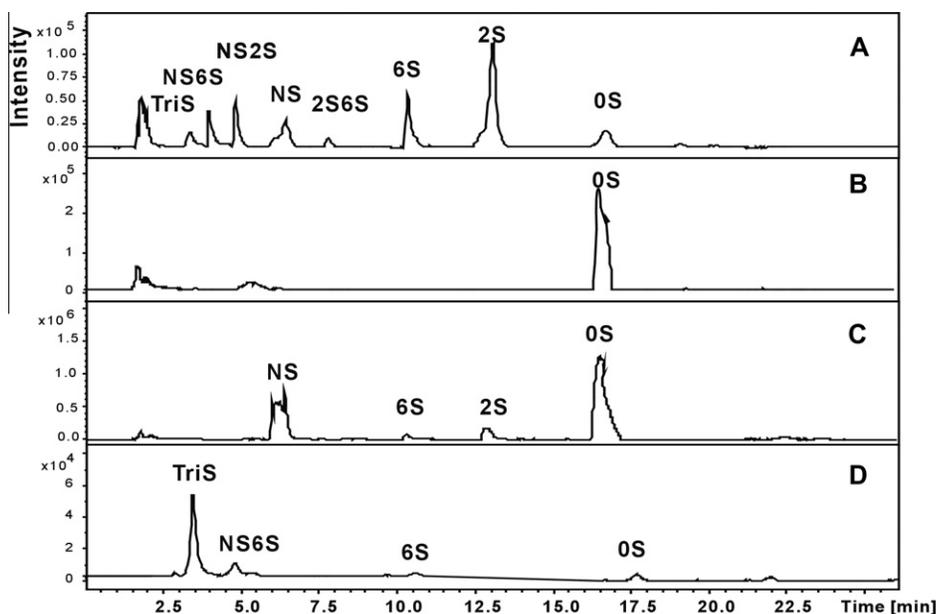
**Fig. 2.** GAGs recovered from CHO-S and MST cells were identified by disaccharide analysis, following AMAC tagging, using RP-HPLC-MS with EIC detection. Buffers A and B were 80 mM  $\text{NH}_4\text{HCO}_3$  and methanol. (A) Eight standard AMAC-disaccharides from HS/HP (disaccharides elute from high to low sulfation). (B) GAGs recovered from CHO cells in 0.6 M NaCl wash. (C) GAGs recovered from CHO cells in 1.0 M NaCl wash. (D) GAGs recovered from MST cells in 1.6 M NaCl wash.
