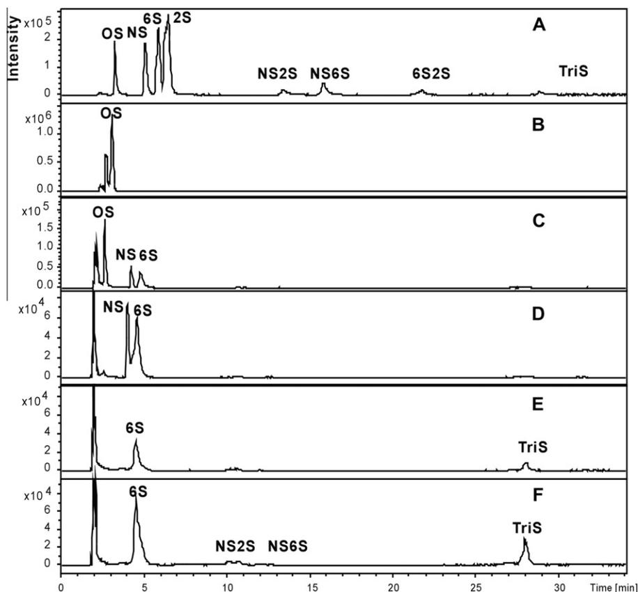
**Fig. 1.** GAGs recovered from a mixture of heparosan, heparan sulfate, and heparin (50 µg of each) and albumin were identified by disaccharide analysis using RP-IP-HPLC-MS with EIC detection. (A) Eight standard disaccharides from HS/HP (disaccharides elute from low to high sulfation). (B) GAGs recovered in 0.6 M NaCl wash. (C) GAGs recovered in 0.8 M NaCl wash. (D) GAGs recovered in 1.0 M NaCl wash. (E) GAGs recovered in 1.2 M NaCl wash. (F) GAGs recovered in 1.6 M NaCl wash.
