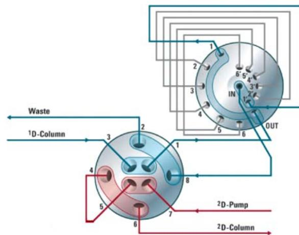
**Figure 1.** Schematic of the loop-based multiple heart-cutting two-dimensional chromatography system.
