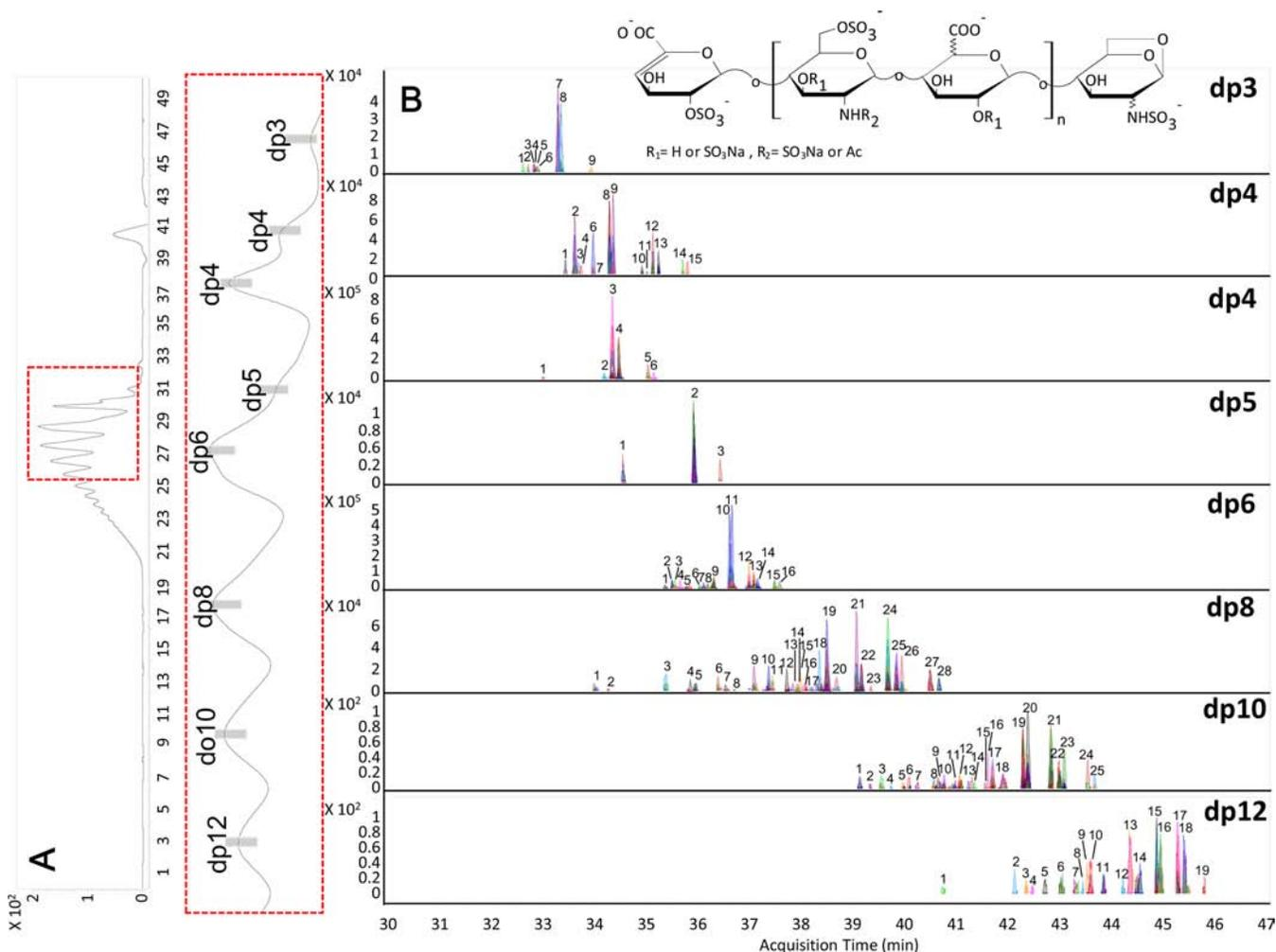
**Figure 3.** Profiling analysis of enoxaparin using MHC-2D-LC-Q/TOF-MS. (A) The first dimensional chromatogram of enoxaparin and the cutting position of each dp from 3 to 12 is shown. (B) The second dimensional chromatograms (ECC) for dp3 to dp12 are shown. In these fractions, the 9 to 28 peaks observed are numbered based on their retention times.
