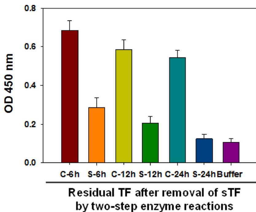
**Figure 5.** Two-step enzymatic oxidation for the separation of TF glycoforms. (A) Removal of sialic acid and oxidation of galactose followed by capture and removal of oxidized sTF. (B) Quantification of two-step enzymatic oxidation for the separation of TF glycoforms.
