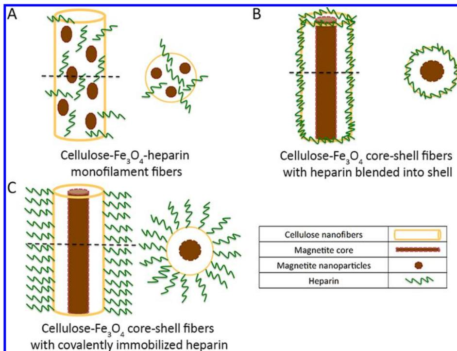
**Figure 2.** Structure of nanofibers. (A) Cellulose-Fe<sub>3</sub>O<sub>4</sub>-heparin monofilament fibers with entrapped Fe<sub>3</sub>O<sub>4</sub> NPs and heparin. (B) Cellulose-Fe<sub>3</sub>O<sub>4</sub> core-shell nanofiber with internal Fe<sub>3</sub>O<sub>4</sub> NP core and cellulose shell blended with heparin. (C) Cellulose-Fe<sub>3</sub>O<sub>4</sub> core-shell nanofiber with internal Fe<sub>3</sub>O<sub>4</sub> NP core and cellulose shell with covalently immobilized heparin.
