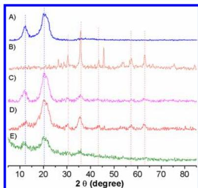
**Figure 8.** XRD spectra of  $\text{Fe}_3\text{O}_4$  NPs and nanofiber composites. A) cellulose nanofibers, B)  $\text{Fe}_3\text{O}_4$  NPs, C) cellulose- $\text{Fe}_3\text{O}_4$  core-shell fibers with immobilized heparin on shell, D) cellulose- $\text{Fe}_3\text{O}_4$ -heparin monofilament fibers, E) cellulose- $\text{Fe}_3\text{O}_4$  core-shell fibers with heparin blended into the shell.
