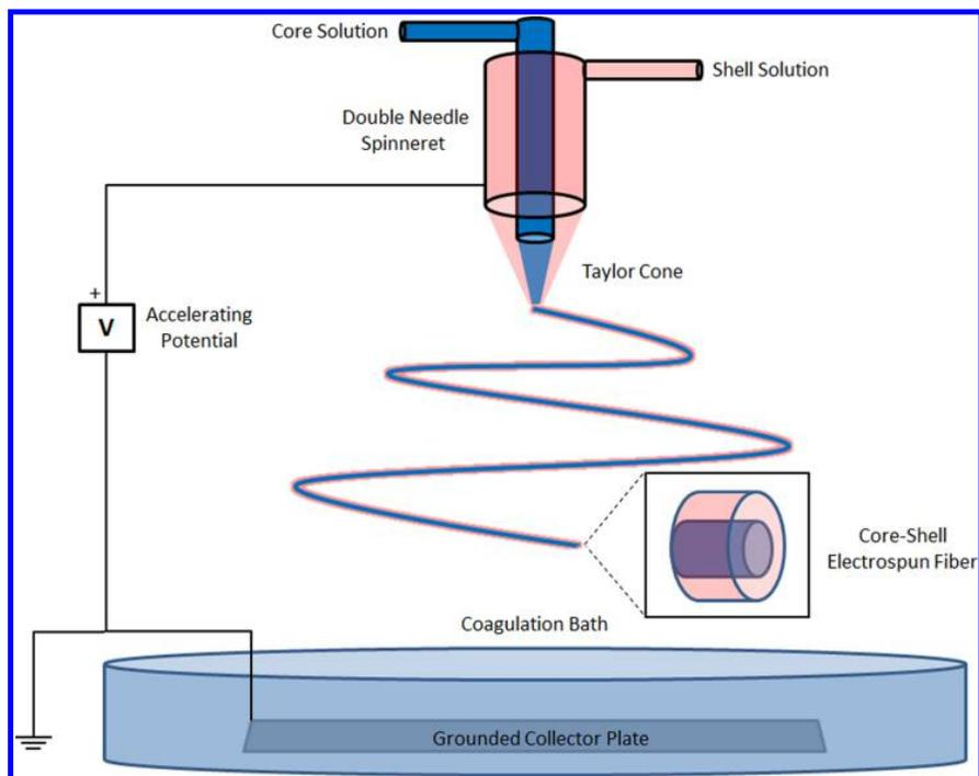
**Figure 1.** Electrospinning of core–shell fibers is accomplished using a coaxial spinneret. Two different solutions are pumped at different rates into the spinneret and accelerated by a potential, forming a Taylor cone and elongating into fibers that are collected in a grounded coagulation bath.
