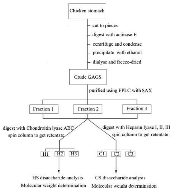
**Fig. 2** Diagram of process flow chart
