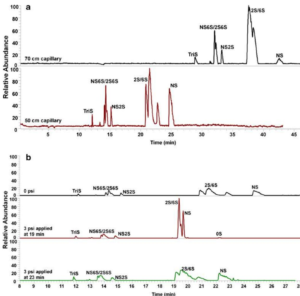
**Fig. 2** Optimization of (a) capillary length and (b) pressure on CE–MS analysis of 8 disaccharide standards. Background electrolyte and sheath liquid, 10 mM ammonium acetate (AA) in 80 % aqueous methanol; separation voltage,  $-30$  kV; electrospray voltage,  $-1.7$  kV
