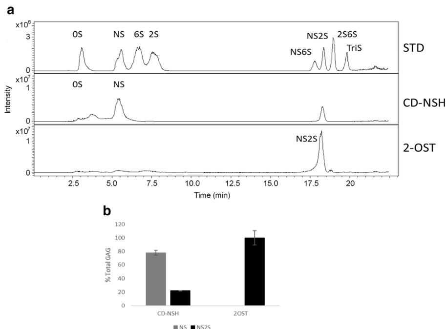
**Fig. 5** LC-MS disaccharide analysis of t6-OST-3 sulfotransferase activity. Standard consists of eight known disaccharides. Error bars are standard deviation of duplicate runs
