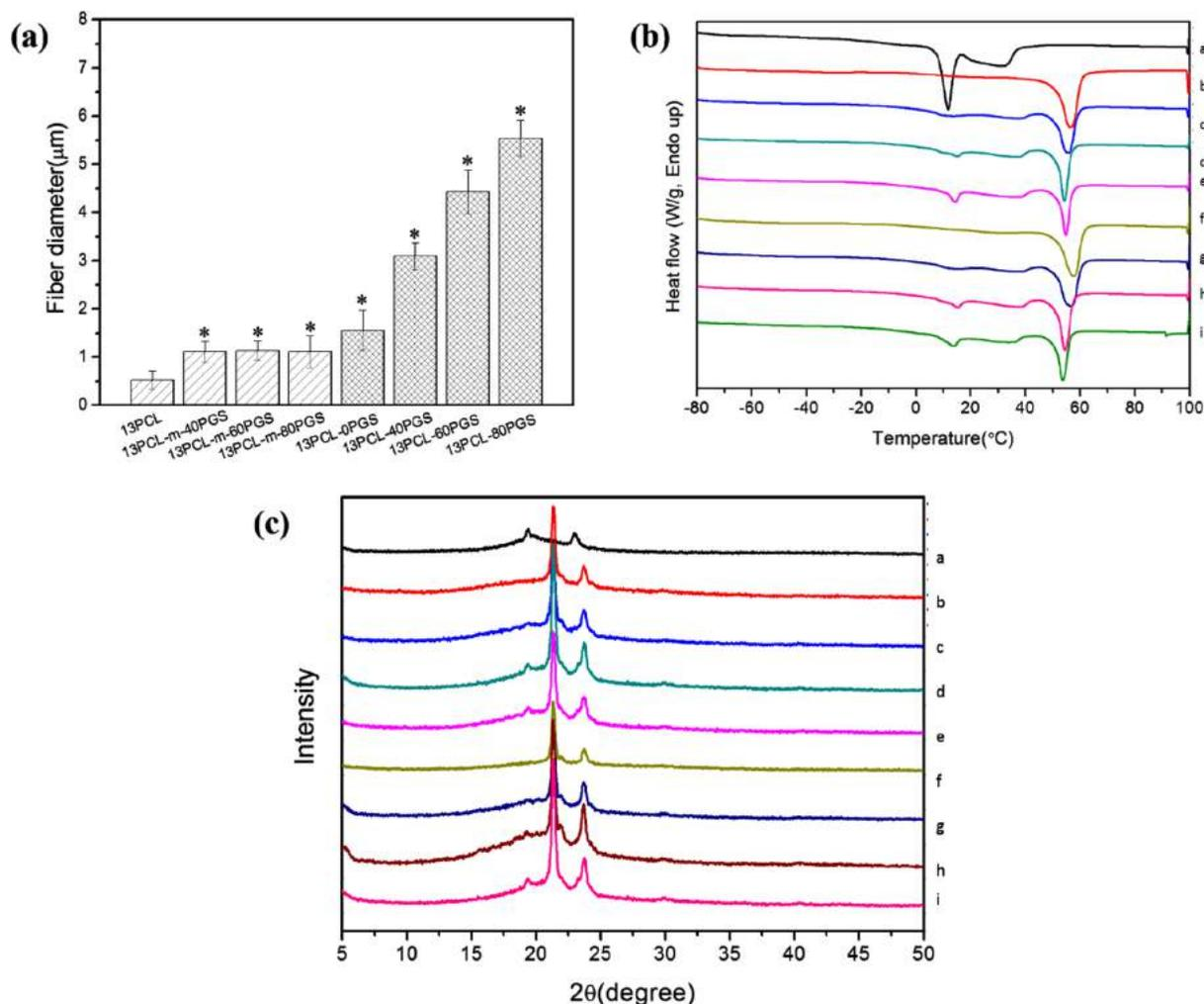
**Figure 3.** (a) Effect of the PCL–PGS ratio on fiber diameter. \*Significance ( $p < 0.05$ ) is based on comparison against 13PCL fiber diameter, and error bars represent the standard deviation. (b) DSC analysis of the sixth cycle of mixture fibers and core–shell fibers. (c) X-ray diffraction spectra for the mixture fibers and core–shell fibers. ((a) PGS, (b) 13PCL, (c) 13PCL–m-40PGS, (d) 13PCL–m-60PGS, (e) 13PCL–m-80PGS, (f) 13PCL–0PGS, (g) 13PCL–40PGS, (h) 13PCL–60PGS, and (i) 13PCL–80PGS).
