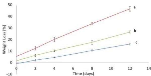
**Figure 5.** Accelerated in vitro degradation (mass loss, %) of (a) 13PCL-m-80PGS, (b) 13PCL-80PGS, and (c) 13PCL in 1 mM NaOH. Error bars represent the standard deviation.
