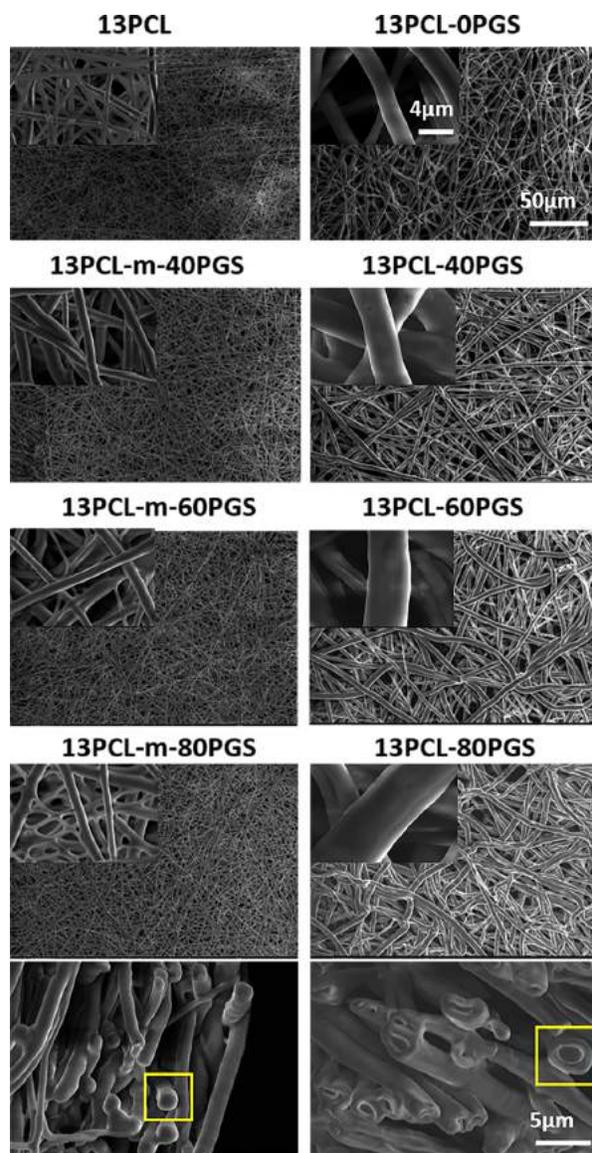
**Figure 2.** SEM images of mixture fibers 13PCL, 13PCL–m-40PGS, 13PCL–m-60PGS, and 13PCL–m-80PGS and core–shell fibers 13PCL–0PGS, 13PCL–40PGS, 13PCL–60PGS, and 13PCL–80PGS at 50 and 4  $\mu$ m. SEM images of cross section for 13PCL–80PGS and 13PCL–m-80PGS at 5  $\mu$ m.
