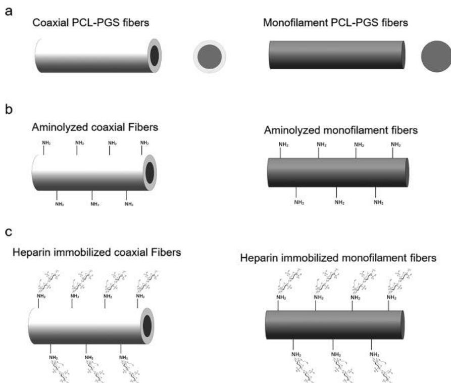
**Figure 1.** Drawing of types of electrospun fibers prepared for the study. NX 10 (version 10, Siemens PLM) was used. (a) Unmodified mono and coaxial PCL–PGS fibers. (b) Aminolyzed mono and coaxial PCL–PGS fibers. (c) Heparin-immobilized mono and coaxial PCL–PGS fibers.
