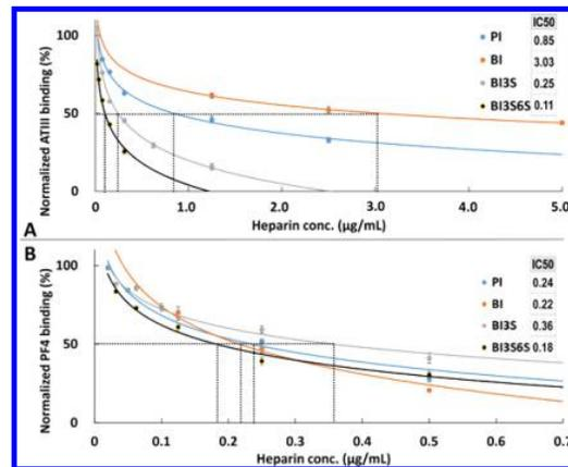
**Figure 4.** Surface plasmon resonance IC<sub>50</sub> measurement of bovine heparins using surface competition SPR: (A) IC<sub>50</sub> for AT binding of heparins; (B) IC<sub>50</sub> for PF4 binding of heparins.
