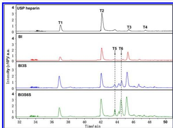
**Figure 3.** Extracted ion chromatogram of tetrasaccharide mapping on BI heparins and PI heparin. T1 ( $m/z$  477) is  $\Delta\text{UA-GlcNAc6S-GlcA-GlcNS3S}$ . T2 ( $m/z$  517) is  $\Delta\text{UA-GlcNAc6S-GlcA-GlcNS3S6S}$ . T3 ( $m/z$  536) is  $\Delta\text{UA-GlcNS6S-GlcA-GlcNS3S6S}$ . T4 ( $m/z$  557) is  $\Delta\text{UA-GlcNAc2S6S-GlcA-GlcNS3S6S}$ . T5 ( $m/z$  536) and T6 ( $m/z$  536) have unknown structures.
