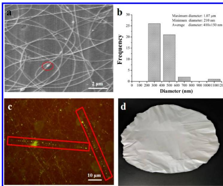
**Figure 5.** SEM image (a), fiber diameter distribution (b), and inverted fluorescence microscope image (c) of the FOS/PVA/*L. plantarum* nanofibrous film (d).
