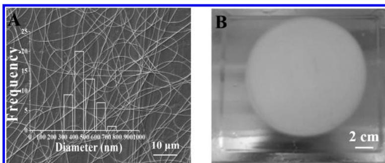
Figure 3. Images of the obtained electrospun 2.5%FOS/6%PVA film ((A) SEM image; (B) deposited on the aluminum foil).
