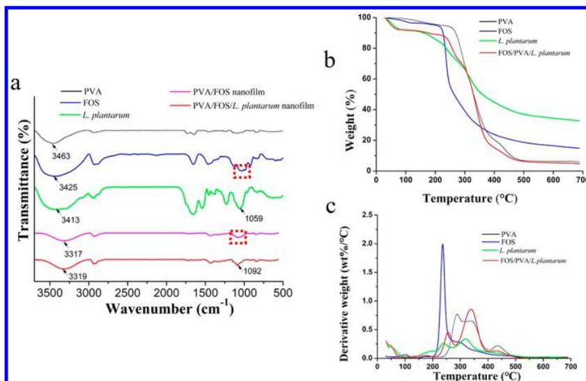
**Figure 6.** FTIR spectra (a), TG (b), and DTG (c) curves of different samples.
