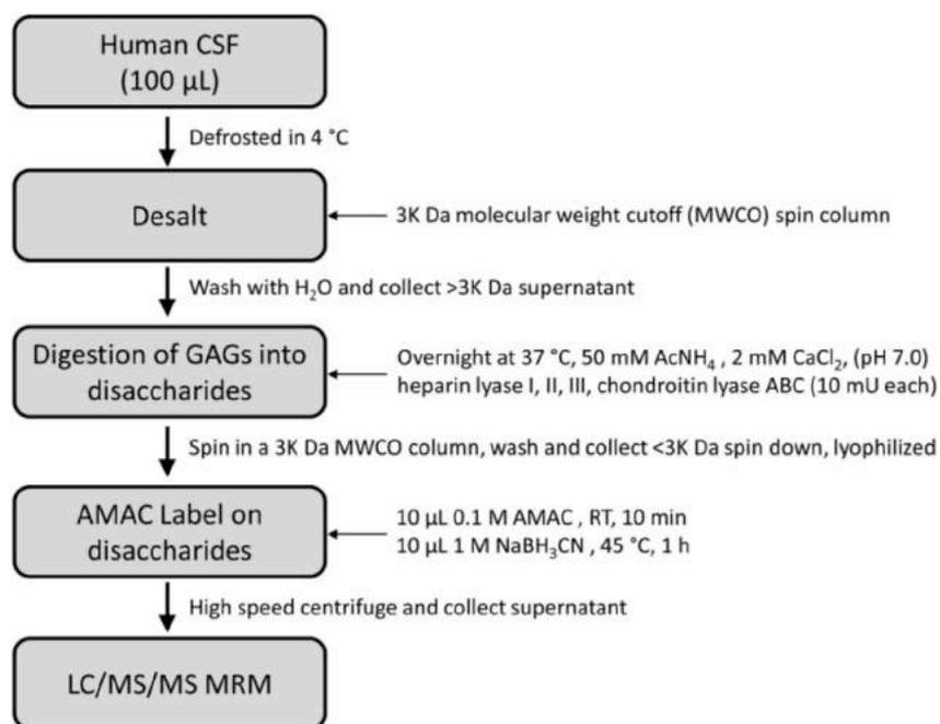
**Fig. 1.** Analytical workflow for quantitative measurement GAG content and composition in human CSF. Excess AMAC is removed as a precipitate in the final step and residual AMAC (eluting as an early peak) is diverted from the mass spectrometer.
