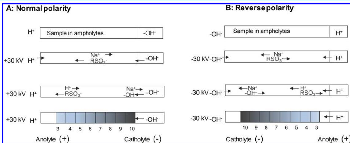
**Figure 1.** Schematic of negative-ion mode cIEF-MS workflow showing both (A) normal polarity and (B) reverse polarity separations.
