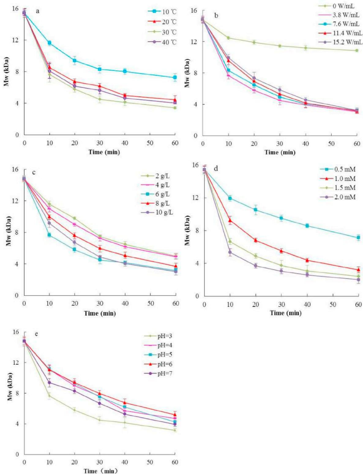
Fig. 2. Effect of different treatment factors on the Mw of heparin. a. temperature; b. ultrasonic intensity; c. H<sub>2</sub>O<sub>2</sub> concentration; d. Fe<sup>2+</sup> concentration; e. pH.
