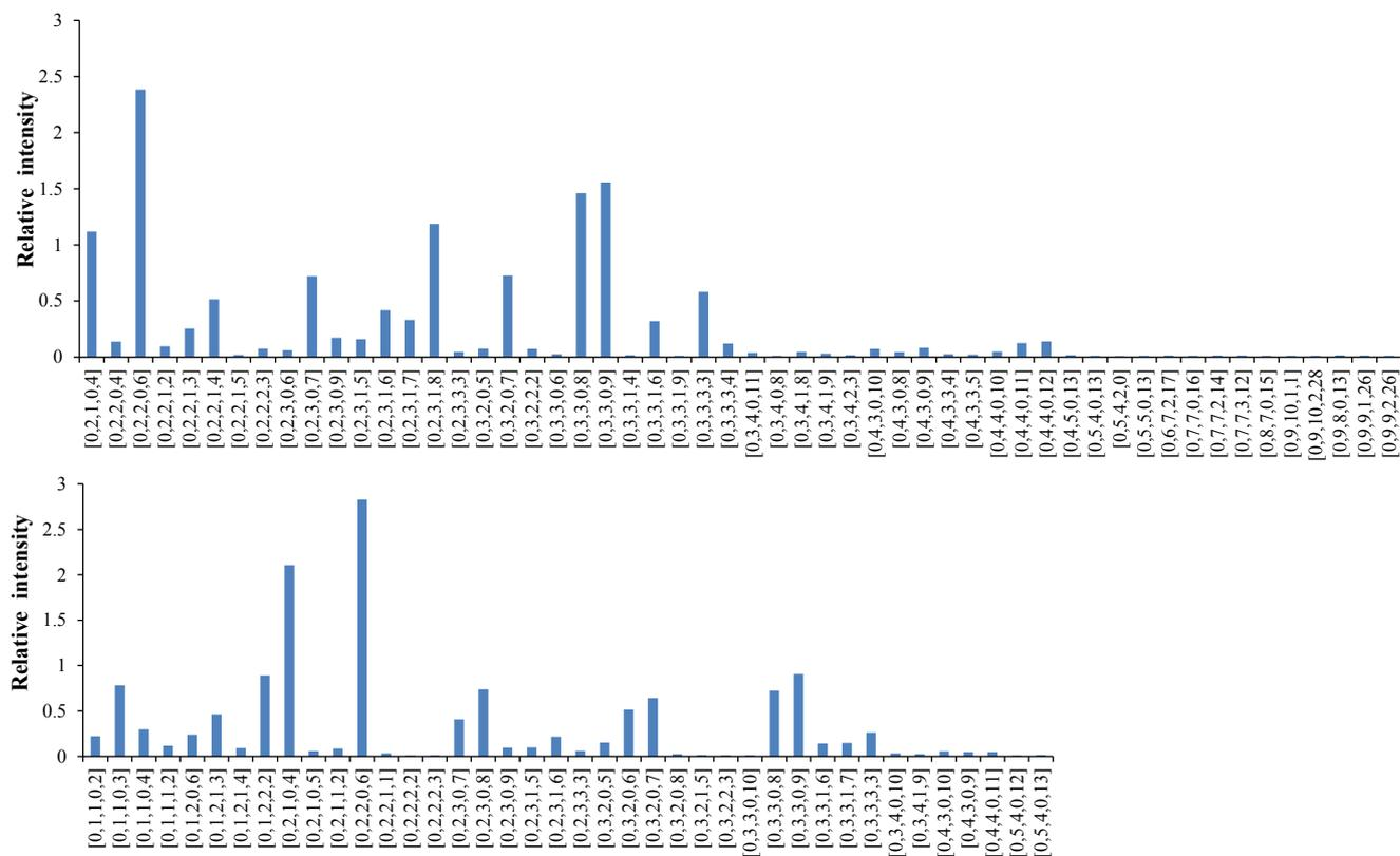
Fig. 6. Top-down approach using HILIC LC-FT-ESI-MS to characterize LMWH-1 and LMWH-4. (a) Detected LMWH-1 oligosaccharides. (b) Detected LMWH-4 oligosaccharides. The oligosaccharides are labeled with the number of [HexA, HexA, GlcN, Ac, SO<sub>3</sub>] moieties present in each structure.
