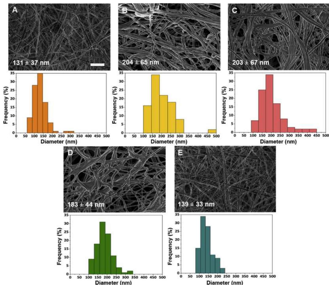
**Fig. 1.** SEM images and respective histograms (below) of PBI electrospun fibers. (A) Neat PBI fibers and fibers treated with (B)  $\text{H}_2\text{SO}_4$ , (C) CSA, (D) HEPES, and (E) NaCl (scale bar = 2  $\mu\text{m}$ ). PBI, polybenzimidazole; SEM, scanning electron microscopy; CSA,  $\beta$ -camphorsulfonic acid; HEPES, 4-(2-hydroxyethyl)-1-piperazineethanesulfonic acid.
