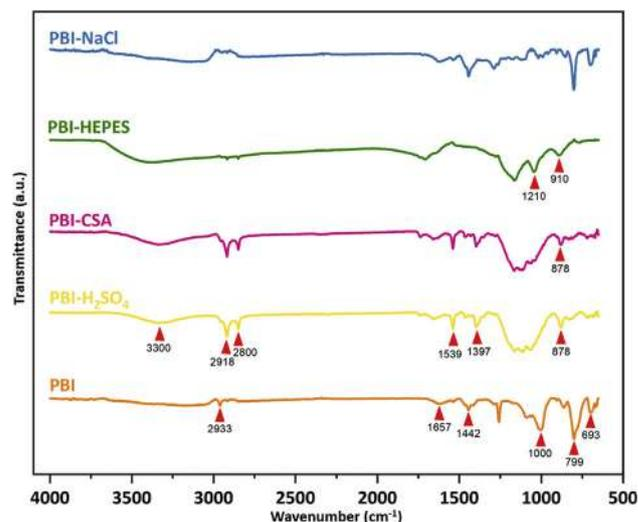
**Fig. 2.** ATR-FTIR profiles (resolution  $4 \text{ cm}^{-1}$ , 32 scans) for PBI fibers with no doping and doped with  $\text{H}_2\text{SO}_4$ , CSA, HEPES, and NaCl. ATR, attenuated total reflectance; FTIR, Fourier-transform infrared spectroscopy; PBI, polybenzimidazole; CSA,  $\beta$ -camphorsulfonic acid; HEPES, 4-(2-hydroxyethyl)-1-piperazineethanesulfonic acid.
