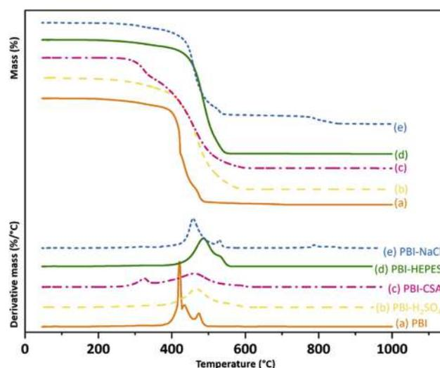
Fig. 3. TGA profiles ( $1.5\text{ }^\circ\text{C per min}$ ,  $150\text{--}1,000\text{ }^\circ\text{C}$ , with 20% oxygen) of PBI electrospun fibers, not doped or doped with  $\text{H}_2\text{SO}_4$ , CSA, HEPES, and NaCl, and respective first derivatives. TGA, thermogravimetric analysis; CSA,  $\beta$ -camphorsulfonic acid; HEPES, 4-(2-hydroxyethyl)-1-piperazineethanesulfonic acid; PBI, polybenzimidazole.
