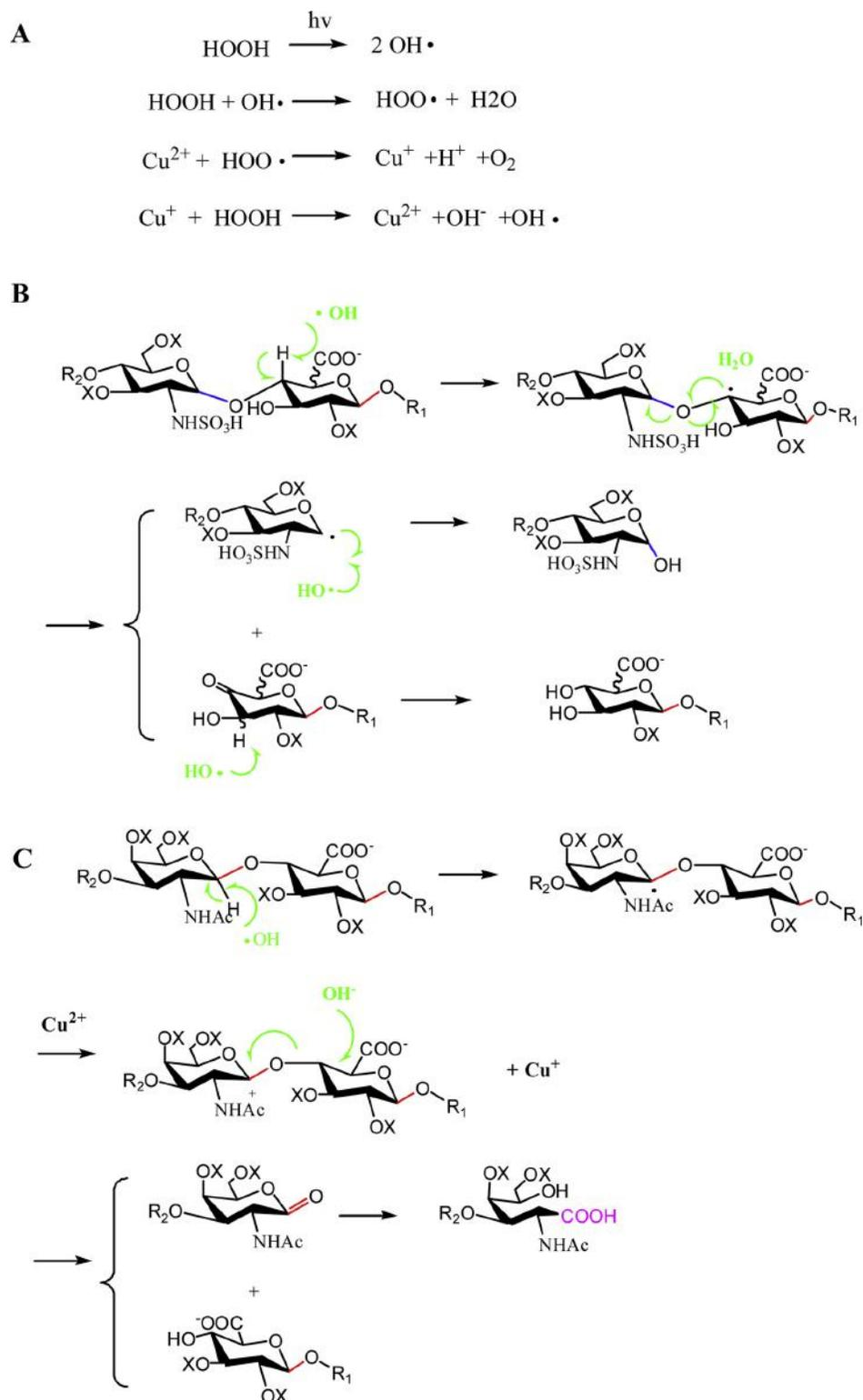
**Fig. 4.** Proposed mechanism for Fenton-type free radical degradation of different GAGs (A. Free radical degradation of GAGs produce most oligosaccharide maintain their basic structural unit. B. Free radical degradation of GAGs (especially the GAGs with  $\beta$ -linked structural units) involves oxidative breaking of glycosidic bonds).
