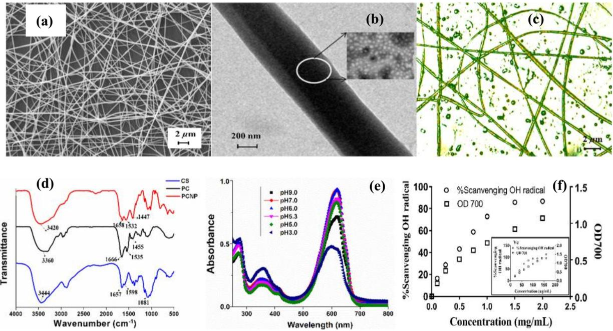
**Fig. 1.** (a) SEM image of PC-loaded EFM containing GOS; (b) TEM image of obtained fiber and PCNP; (c) CLSM image of obtained fiber (d)FTIR spectra of different sample; (e) absorption spectrum of PC under different pH; (f) antioxidant activity of different concentrations of PC-loaded EFM containing GOS.
