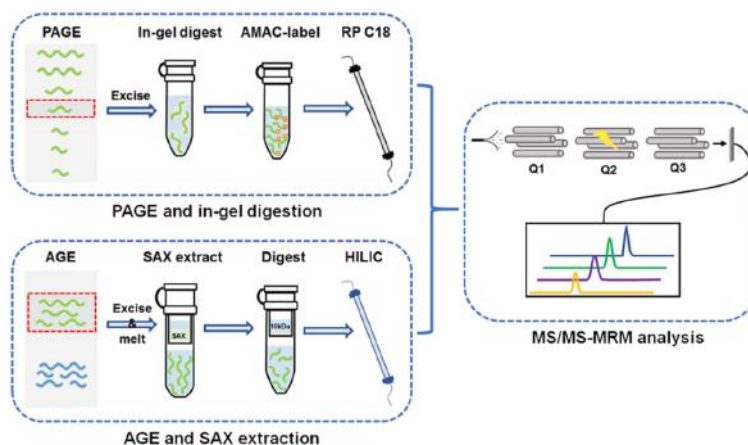
Figure 3. Analytical workflow for the electrophoresis–MS analysis of GAGs.
