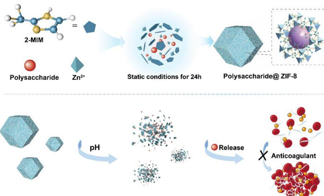
Scheme 1. Schematic representation of the synthesis of polysaccharides@ZIF-8 biocomposites.
