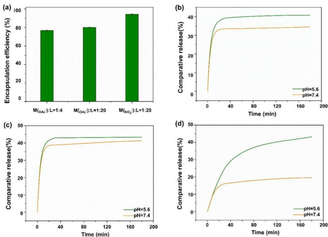
Fig. 3. (a) The encapsulation efficiency of the HP@ZIF-8 synthesized by different zinc precursors and varying metal to ligand ratio. Release profiles of HP@ZIF-8 (b)  $M(OAc^-):L=1:4$ ; (d)  $M(OAc^-):L=1:20$ ; (f)  $M(NO_3^-):L=1:20$ .
