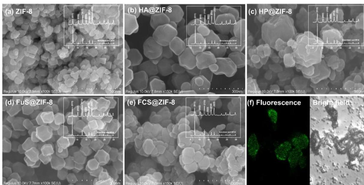
**Fig. 5.** SEM images and XRD patterns of (a) ZIF-8, (b) HA@ZIF-8, (c) HP@ZIF-8, (d) FuS@ZIF-8, (e) FCS@ZIF-8; (f) CLSM images showing the fluorescence and bright-field images of HA@ZIF-8.
