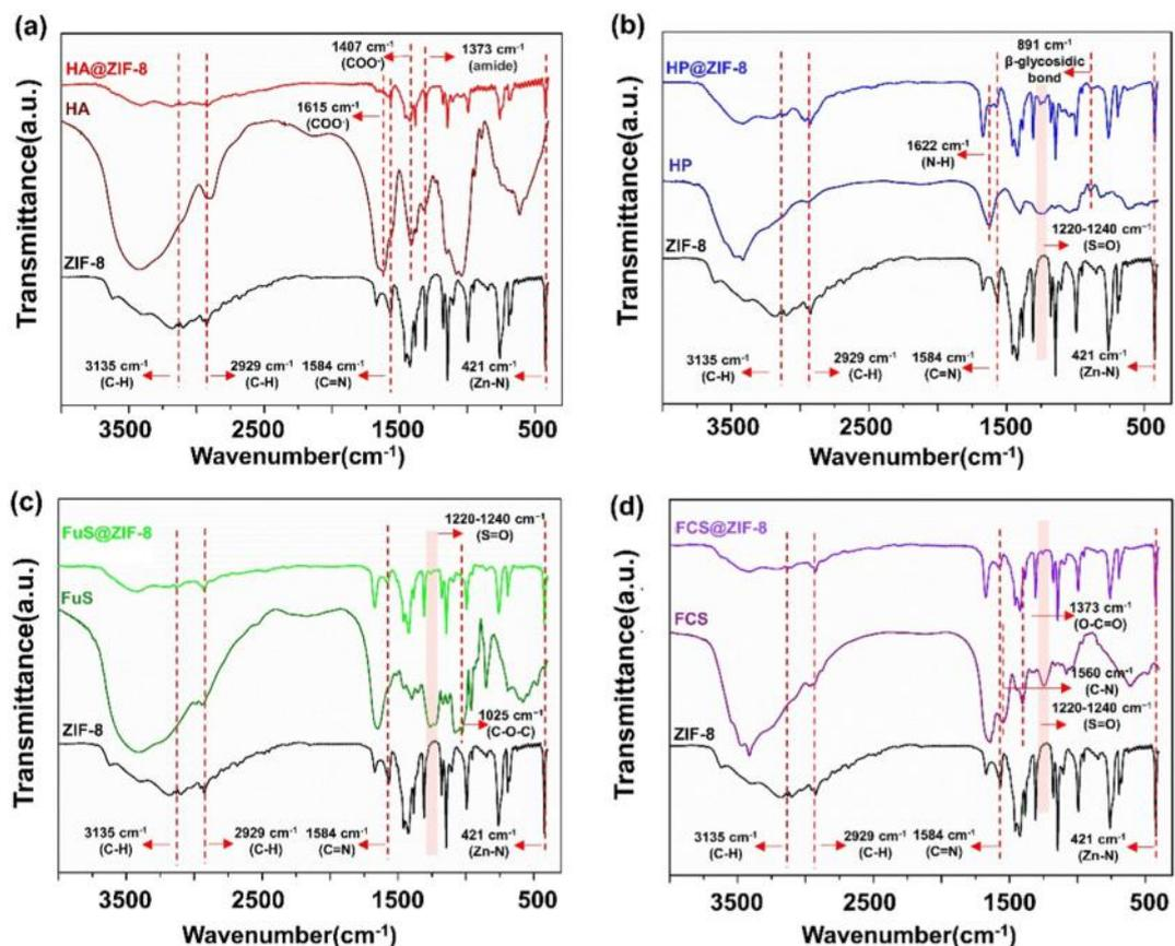
Fig. 4. The FTIR spectra of (a) ZIF-8, HA and HA@ZIF-8, (b) ZIF-8, HP and HP@ZIF-8, (c) ZIF-8, FuS and FuS@ZIF-8 (d) ZIF-8, FCS and FCS@ZIF-8.
