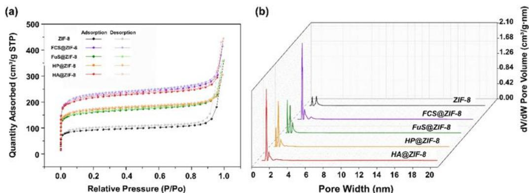
**Fig. 6.** (a) N<sub>2</sub> adsorption isotherms of ZIF-8, FCS@ZIF-8, FuS@ZIF-8, HP@ZIF-8, HA@ZIF-8; (b) the inset shows the BJH pore size distribution curve.
