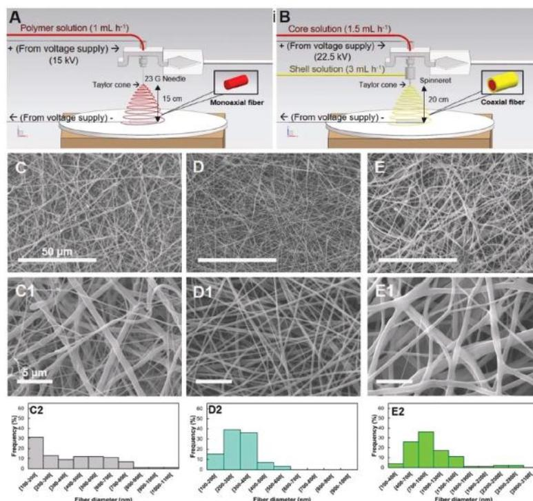
**Fig. 1** Schematics of the electrospinning setups used for the production of (A) monoaxial and (B) coaxial fibers. PCL (C1 and C2), PCL-PANI (D1 and D2) and PGS/PCL-PANI 13% electrospun fibers (E1 and E2), and respective histograms (C3, D3 and E3) ( $n = 100$ ).
