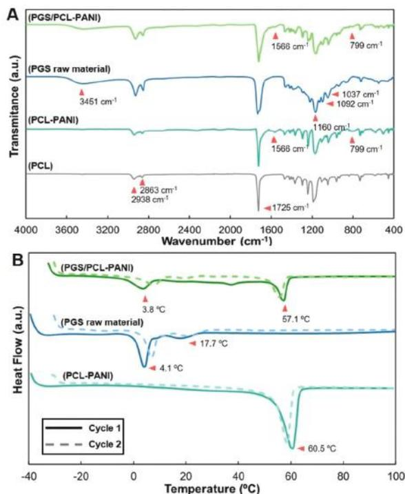
**Fig. 3** (A) ATR-FTIR Spectra for (top to bottom) PGS/PCL-PANI coaxial fibers, PGS raw material, PCL-PANI monoaxial fibers and PCL fibers. (B) Thermograms (heating cycles) of (top to bottom) PGS/PCL-PANI coaxial fibers, PGS raw material and PCL-PANI monoaxial fibers.
