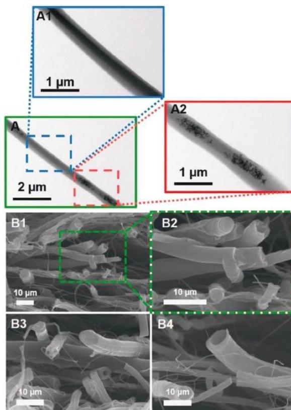
Fig. 2 (A) TEM image of a PGS/PCL-PANI fibers and magnification of two different areas (A1 and A2), using colloidal TiO<sub>2</sub> as the contrast. (B1–4) SEM images of PGS/PCL-PANI coaxial fibers cross-sections.
