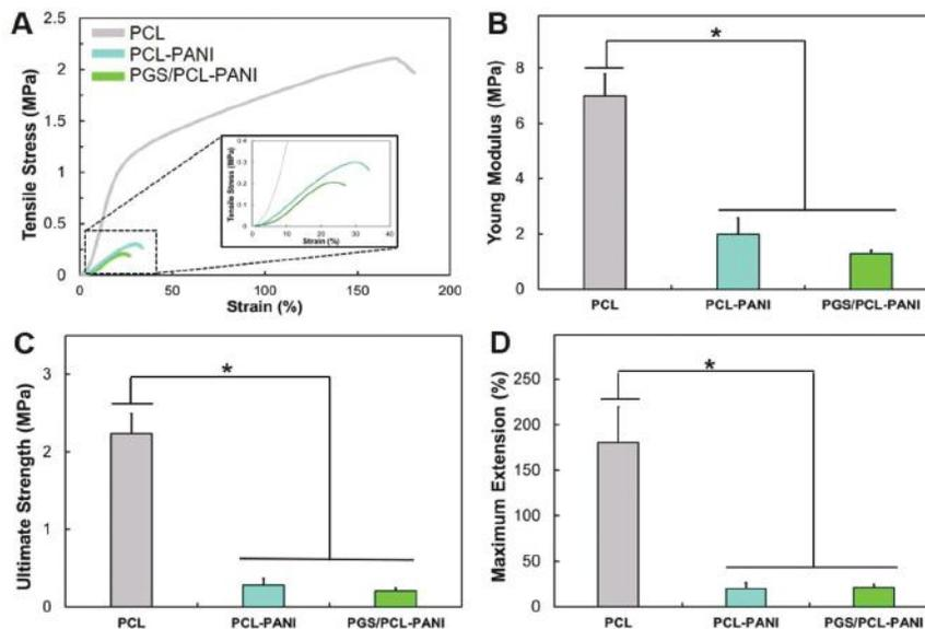
**Fig. 4** Mechanical properties of PCL, PCL-PANI and PGS/PCL-PANI fibers: (A) stress–strain curves for the samples tested; (B) Young's tensile modulus, (C) ultimate strength and (D) maximum extension (\* means  $p < 0.05$ ) (mean  $\pm$  std,  $n = 6$ ).
