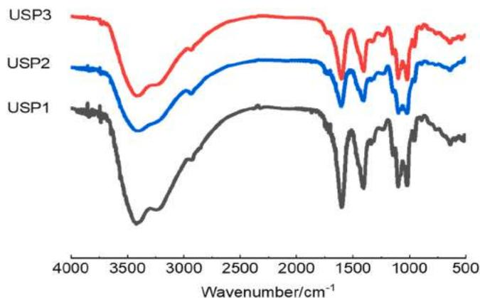
**Fig. 2.** IR spectra (% transmittance as a function wavenumber) of USP1, USP2, and USP3.
