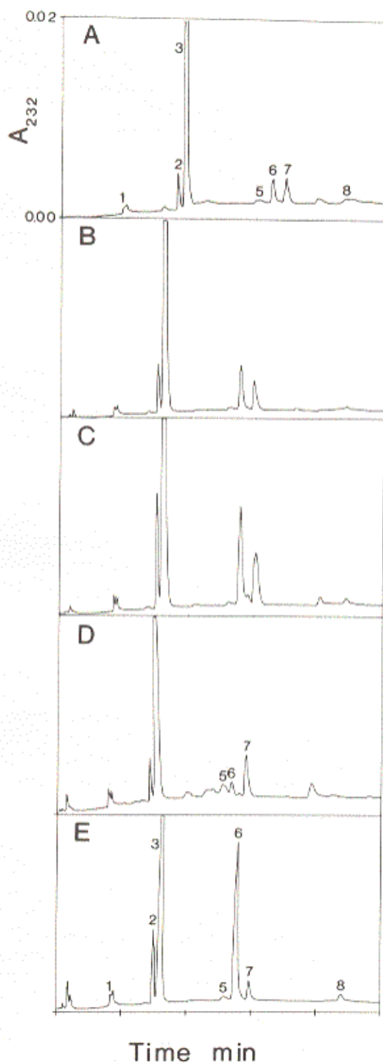
FIG. 4. SAX-HPLC analysis of chondroitinase ABC depolymerized dermatan sulfates. A is dermatan sulfate (E. Coyne). B is size fraction 5 (Fig. 1). C is size fraction 1 (Fig. 1). D is charge fraction 1 (Fig. 2). E is charge fraction 5 (Fig. 2). The tick-marks on the X-axis are at 10-minute intervals.
